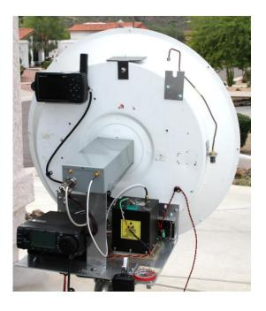
2nd rig Showing packaging, IC-706 Radio Rubidium Standard and a GPS for maidenhead grid during portable operation. Also 2010.
