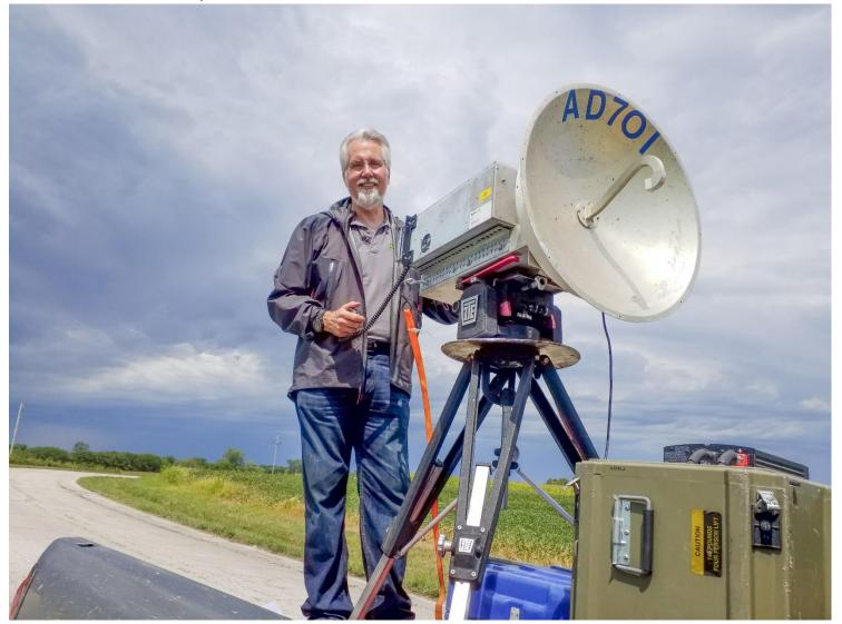
AD7OI using the 2ft dish and 40W rig. Keeping the dish small had advantages for covering the rig during the frequent rains.
