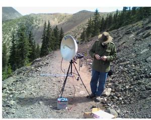
2<sup>nd</sup> rig Based on Kuhne Transverter, 2 Watts TX, LNF LNA and 2ft dish. 2010. Light weight version being operated from 11,300 ft Had to hike the dish to this elevation.
