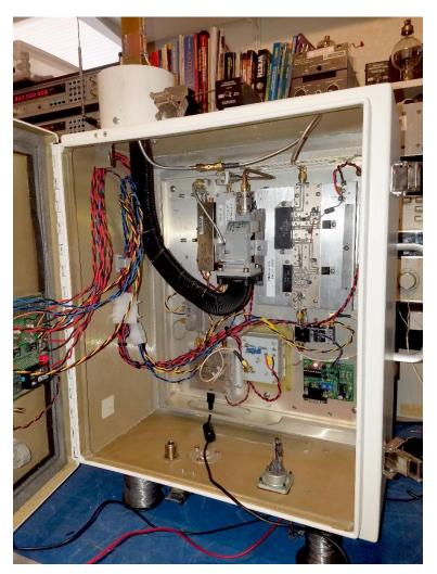
All beacon electronics in an MA COMM repurposed "White Box" Only power is provided up the tower on a single coax.
