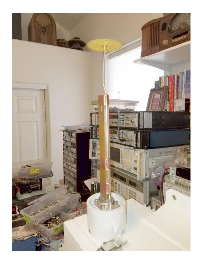
10 GHz Slotted Waveguide Antenna and WA5VJB 1296 "Big wheel" PWB antenna
