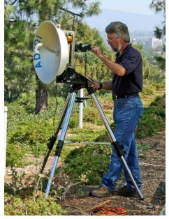
1st rig Based on MA-COM Whitebox parts 90 mW TX and 2ft dish. 2009
