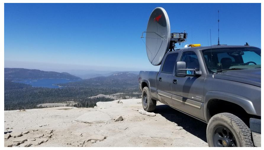
4<sup>th</sup> Generation Truck Mounted AD7OI station using the 6ft dish and a 50W TWT. Total EIRP = 1.02 MW From Bald Mountain Lookout above Shave Lake, Ca. Elev 7730 feet
